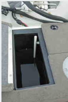
The live wells are seamless roto-molded, which offer leak free performance, optimally placed aerators, and ease of draining and cleaning.
