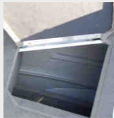
MirroCraft boats have a spray in liner which quiets the hull, eliminates mildew and offers a durable storage area!
